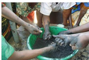
Fig. 13. Molding the mixture into briquettes
